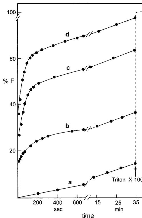
**Figure 6.** Time course of the fluorescence increase when CF-loaded vesicles of sonicated **1** ([**1**] = 1.1 × 10<sup>-4</sup> M, pH 7, 25 °C) are exposed to different concentrations of added TMED C<sub>16</sub>. The arrow indicates when an excess of Triton X-100 was added. ([TMED C<sub>16</sub>] = 0 (a), 1.3 × 10<sup>-5</sup> (b), 2.7 × 10<sup>-5</sup> (c), and 3.3 × 10<sup>-5</sup> M (d).
