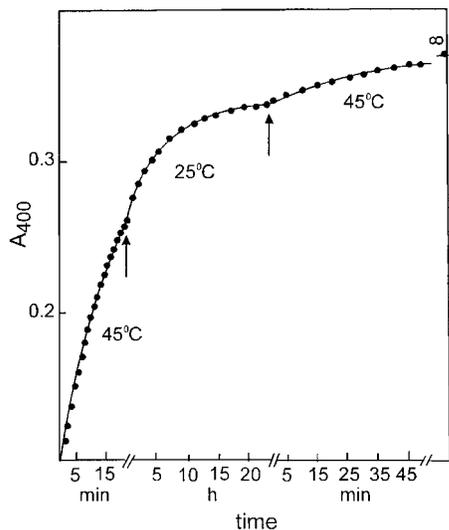
**Figure 3.** Time course of the absorbance at 400 nm of an experiment carried out at different temperatures with sonicated vesicles of  $5.4 \times 10^{-5}$  M lipid **1** and  $1.7 \times 10^{-3}$  M  $\text{EuCl}_3$ . The arrows denote the times of changes of temperature. (Note the changes in the time scale.)
