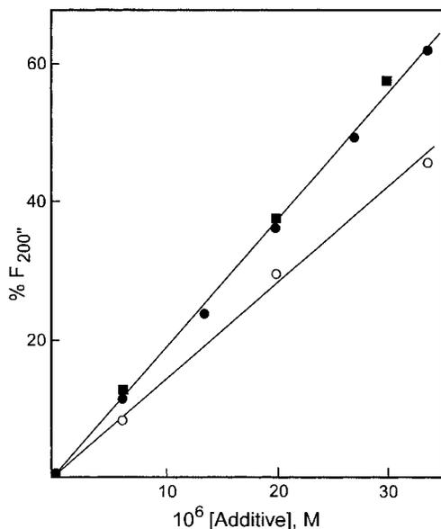
**Figure 7.** Relative amount of released CF after 200 s from CF-loaded vesicles of **1** ([**1**]  $1.1 \times 10^{-4}$  M, pH 7, 25 °C) as a function of the concentration of added TMED C<sub>16</sub> (●), CTABr (■), or C<sub>16</sub>NH<sub>2</sub> (○).
