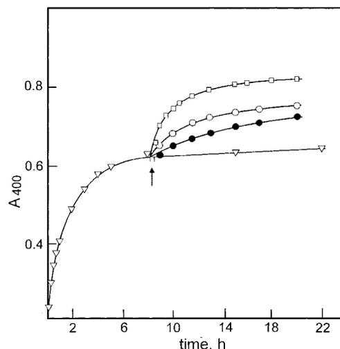
**Figure 5.** Time course of the absorbance at 400 nm for the cleavage of extruded vesicles of  $7.0 \times 10^{-5}$  M lipid **1** upon the addition of  $1 \times 10^{-3}$  M  $\text{TmCl}_3$  (25 °C, pH 7.2, 0.025 M HEPES buffer, 0.025 M KCl). After 8 h (arrow),  $2.5 \times 10^{-5}$  (●),  $5.0 \times 10^{-5}$  (○),  $1.0 \times 10^{-4}$  (□), or no TMED  $\text{C}_{16}$  (▽) was added.
