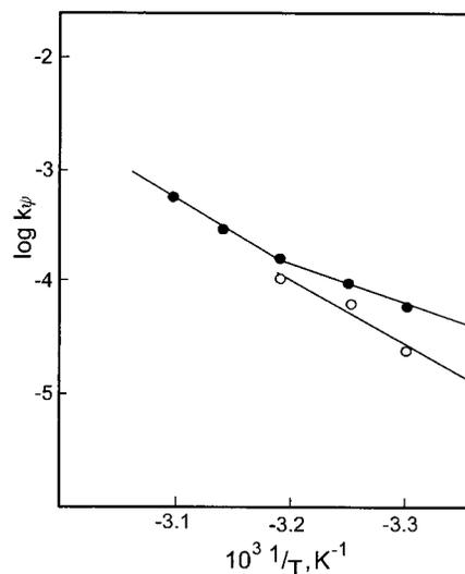
**Figure 2.** Dependence of the observed rate constant,  $k_p$ , for the cleavage of **1** at pH 7 on the inverse temperature. (●) Exovesicular (below  $T_c$ ) or total (above  $T_c$ ) cleavage upon the addition of  $1.7 \times 10^{-3}$  M  $\text{EuCl}_3$  to sonicated vesicles of  $5.4 \times 10^{-5}$  M lipid **1**; (○) endovesicular process in exo-cleaved vesicles upon the addition of  $1.6 \times 10^{-5}$  M TMED  $\text{C}_{16}$ .
